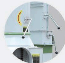
The handle can adjust air volume conveniently
