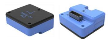
The AHRS-21 is a high-precision, compact, and low-power nine-degree-of-freedom attitude sensor, integrating a six-axis MEMS IMU with a three-axis magnetometer. It provides real-time 3D attitude angles—pitch, roll, and yaw—along with true north heading, using an embedded quaternion-based algorithm and extended Kalman filter for accurate and reliable measurements.
