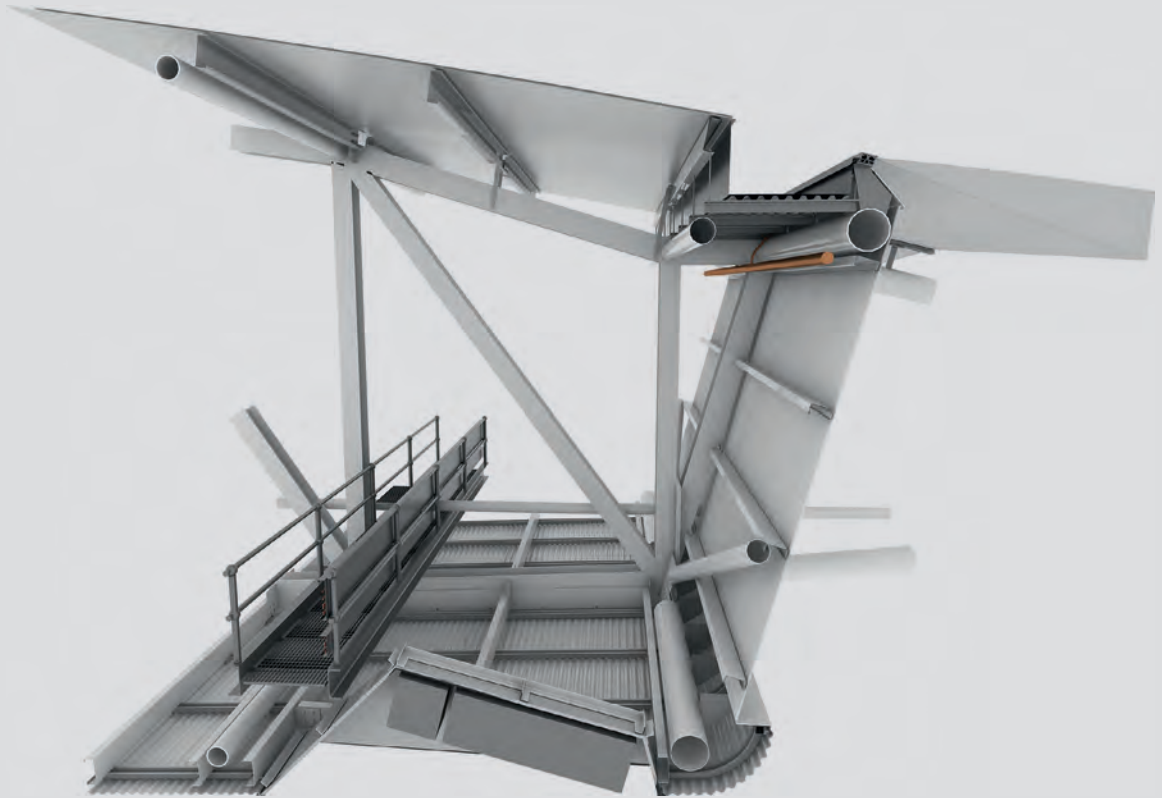
Figure 1-2 Detailed facade systems generated via BIM and visualized as a 3D rendering by COX Architects.
