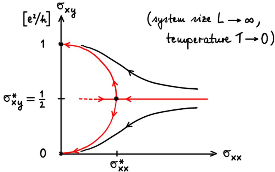
Is this the renormalization group flow diagram for a nonlinear  $\sigma$ -model (Pruisken, 1983) with RG-beta vector field
