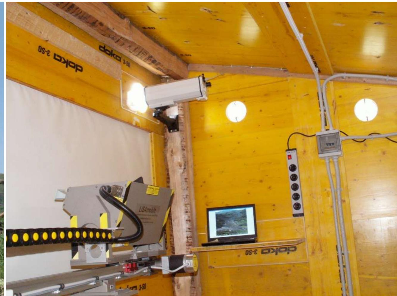
GB-InSAR, LIDAR, thermal and optical imaging
