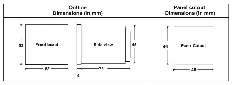
2. Remove the clamp from the controller and push the controller into the panel cutout. Insert the clamp from the rear side until the main is securely fit into the panel.
