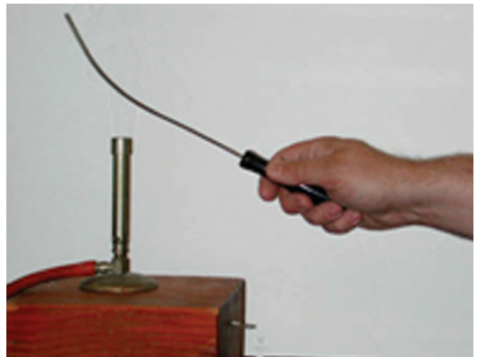
Sumber: www.physics.upenn.edu Gambar 4.6 Saat dipanaskan, bimetal melengkung.
