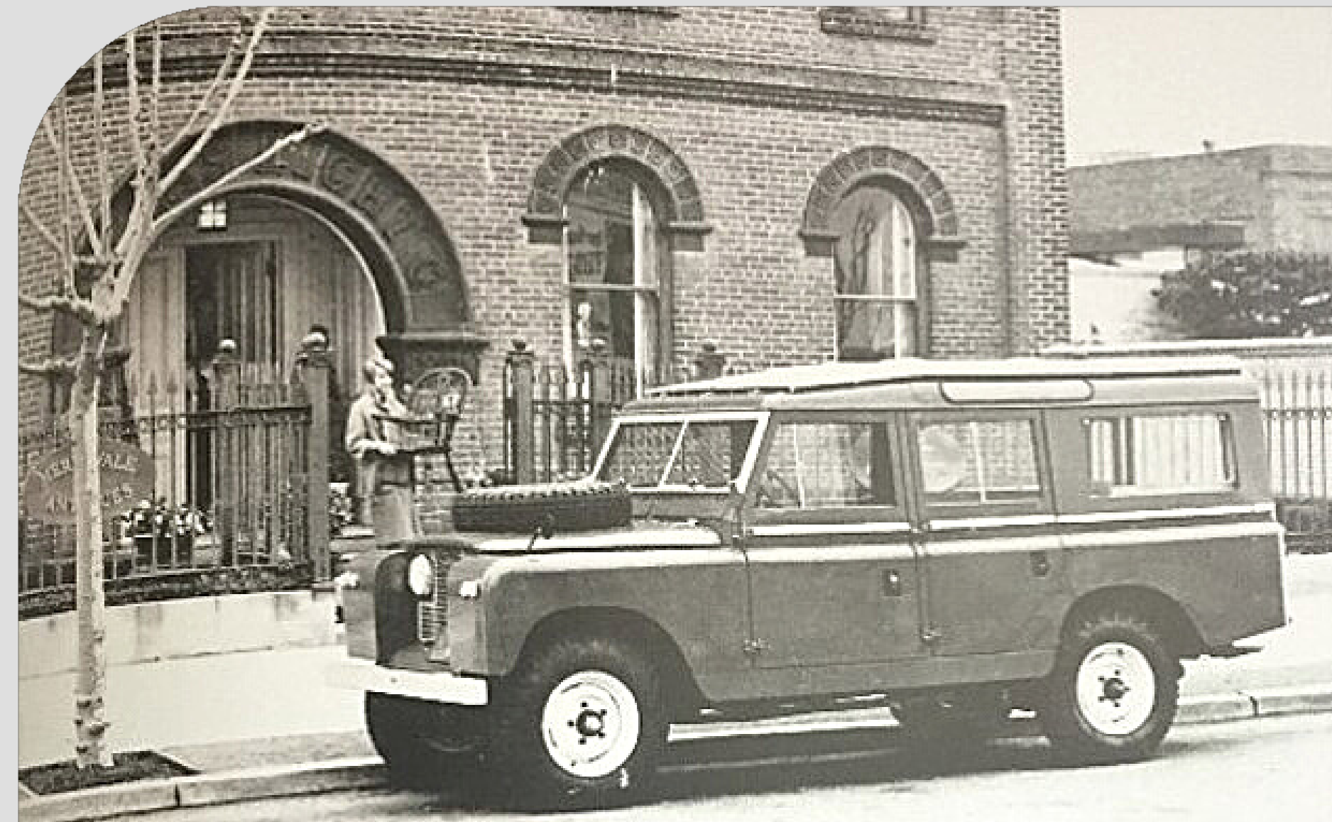
Land-Rover 200 Station Wagon with Heat Shield Roof
