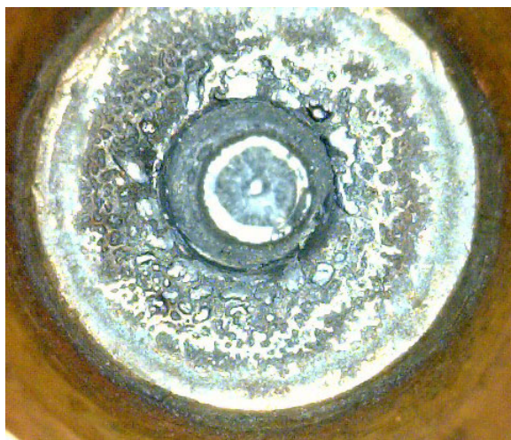
Figure 62 – Non-symmetrical, rough-edged pit and rough-surfaced electrode face
