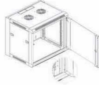
Install front door.
