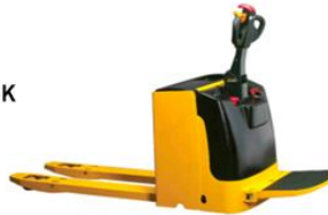
BATTERY OPERATED STACKER PLE - 3130 / STR Capacity - 2000 kg.
