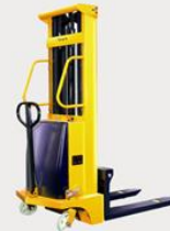
BATTERY OPERATED STACKER PLE - 3130 / STR Capacity - 2000 kg.
